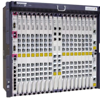
Figure 2.14: Optical Line Terminal (OLT) (Telecomlead, 2017).
