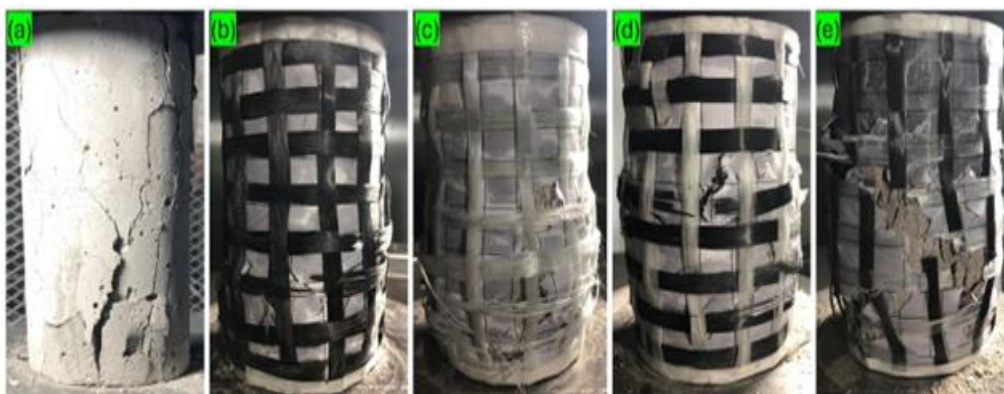
Figure 5 Failure morphology. (a)PC, (b) PWF-C, (c) PWF-G, (d) PWF-C-H, (e) PWF-G-H
