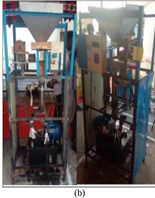
Figure 8: Working prototype of smart and integrated brick making machine
