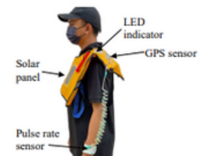
Figure 3. Complete life jacket embedded with sensors
