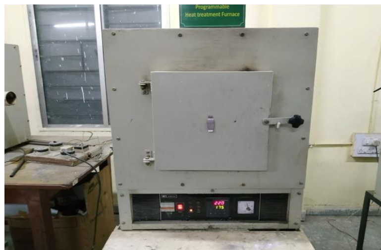
Figure 2 Programmable muffle furnace used for heat treatment
