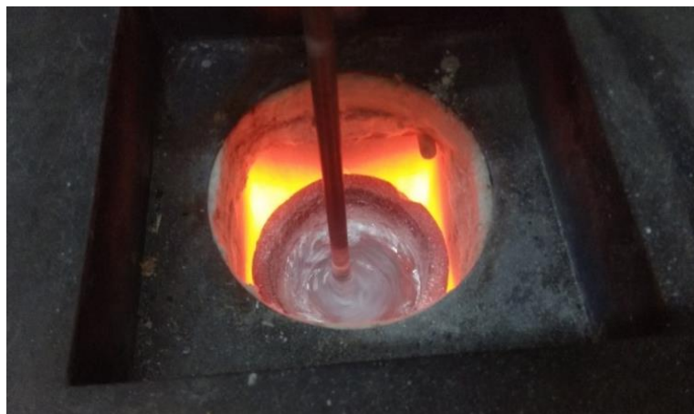
Figure 1 Preparation of sample in Muffle furnace
