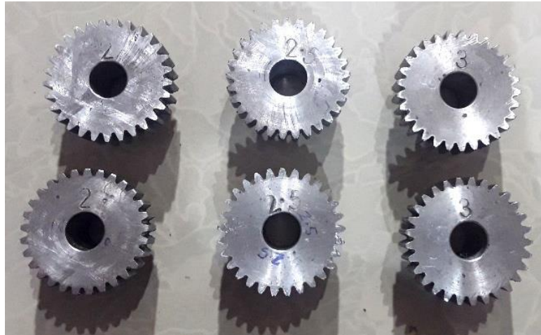
Figure 3. Manufactured Al-nano Al 2 O 3 composite spur gears
