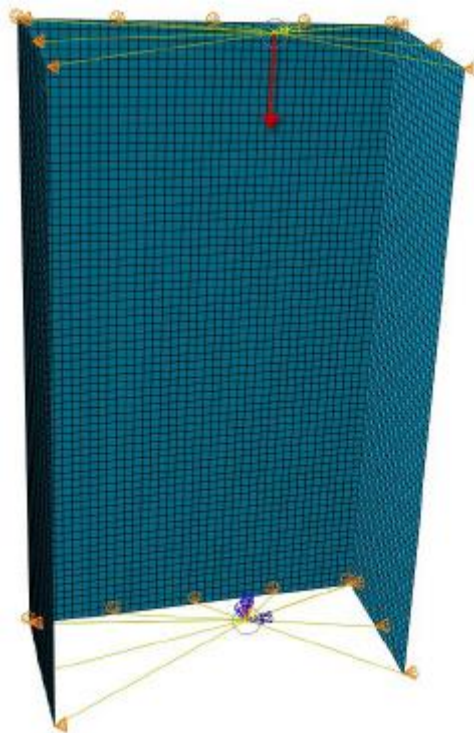
Figure 2. (Pawel Wysmulski) Numerical model FEM during an eccentric compressive load analysis e = 10\text{mm}
