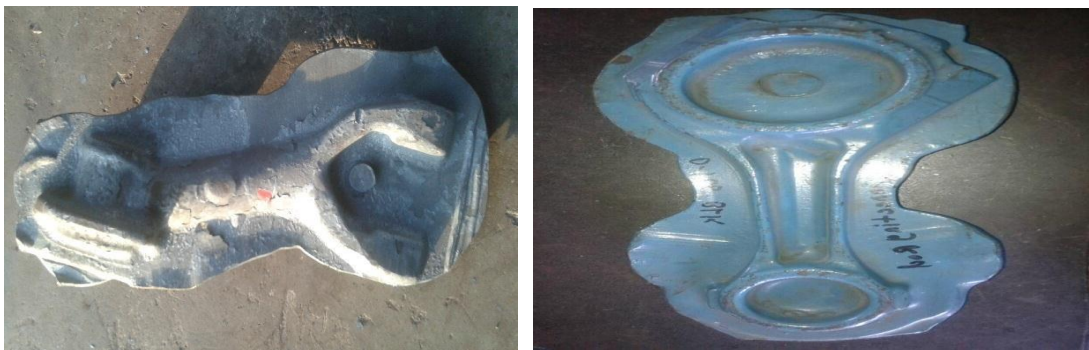
Fig 08 Flash Formation Around Job.
