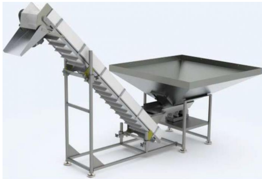
Figure 4c(ii): Hopper with belt conveyor
