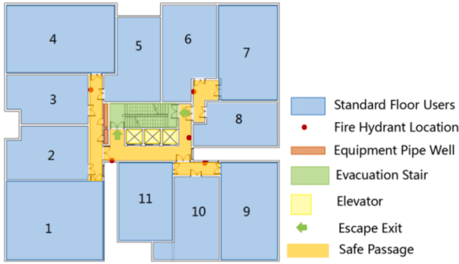
Fig. 10. Standard floor information analysis diagram and BIM model.
