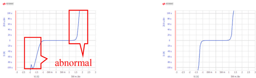
(a) The pin7 to pin8 of the faulty circuit (b) The pin7 to pin8 of the qualified circuit
