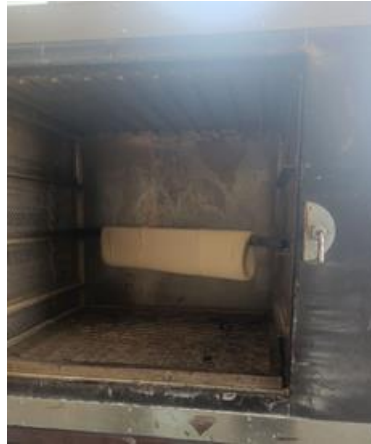
Figure 3 The cast is mounted in the oven with a stocking on.
