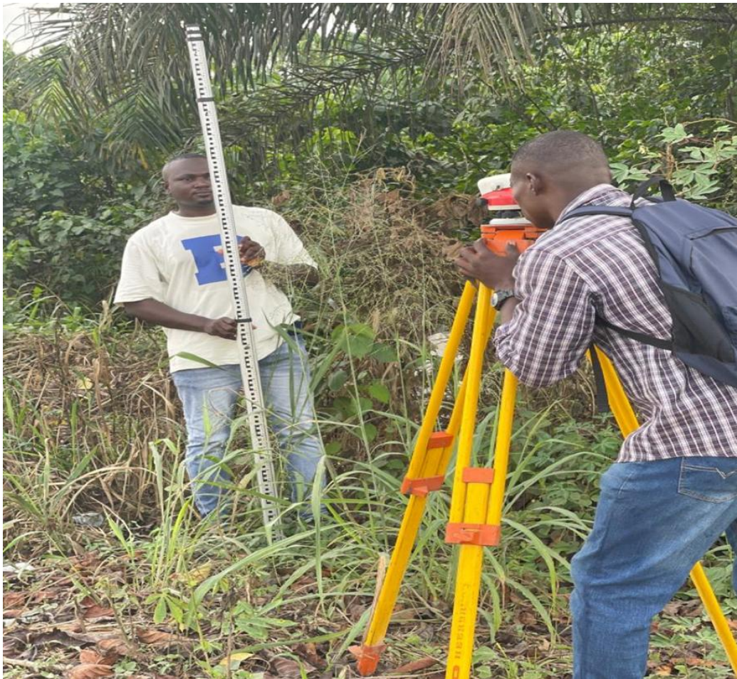
Figure 2.2 – Data Collection using Total Station
