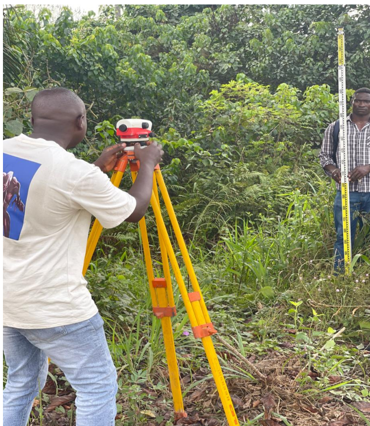
Figure 2.1 – Process of Traversing using leveling instrument
