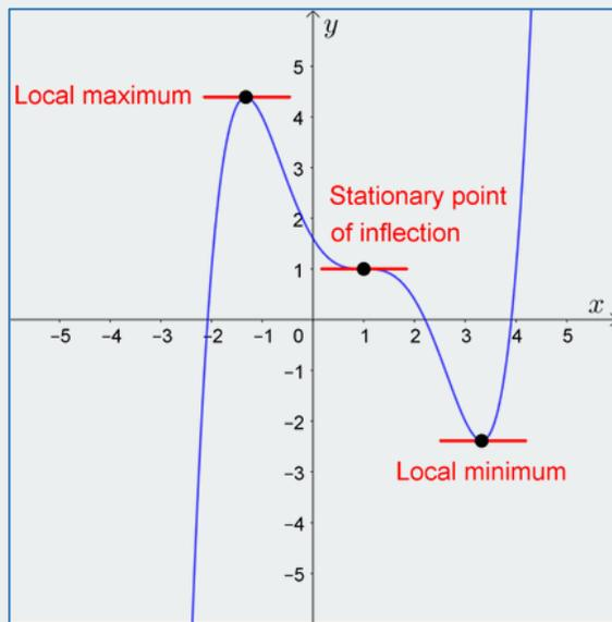
Step to determine the coordinate of stationary point  $y = f(x)$
