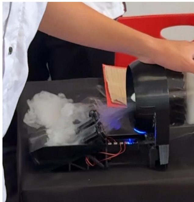
Figure 4.8: The mists got sucked into the Compressor through the six stage of rotors and stator blades
