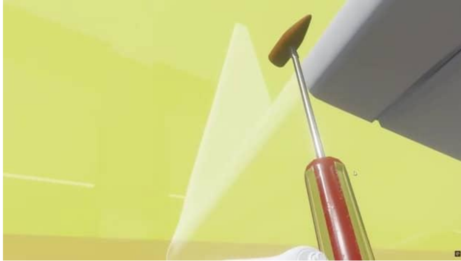
Figure 3.28: Tap Test Hammer Prototype
