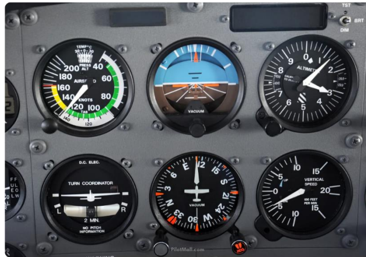
Figure 1.1: Airplane Standard Flight Instrument (istockphoto.com Dec. 29 2009)
