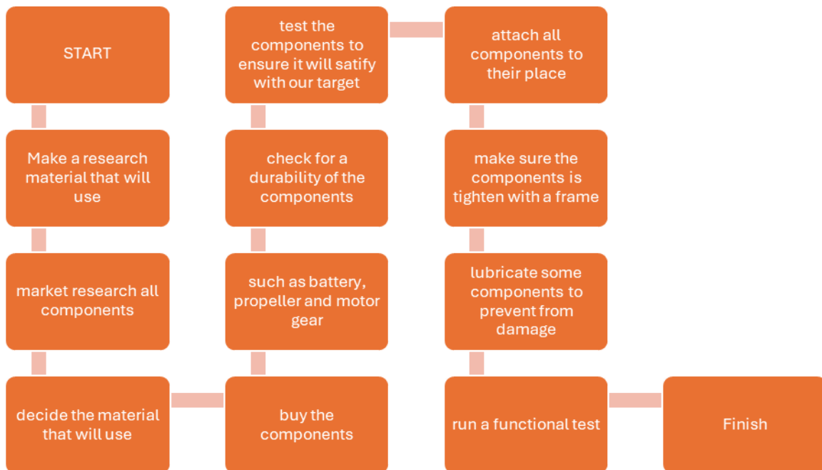
Figure 3.3 Product Mechanisms Design Flow
