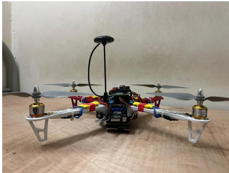
Figure 4.10: Drone with camera below the structure
