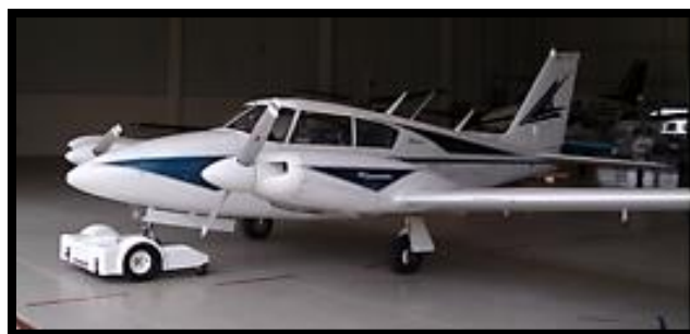
Figure 2.32: Operation of SMARTug on lightweight aircraft (Smarttug.com, n.d.)
