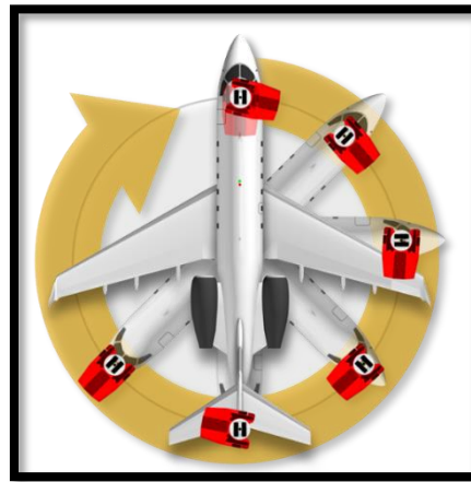
Figure 2.9: shows the flexibility to turnaround the aircraft using remote control aircraft tug (google, n.d.)
