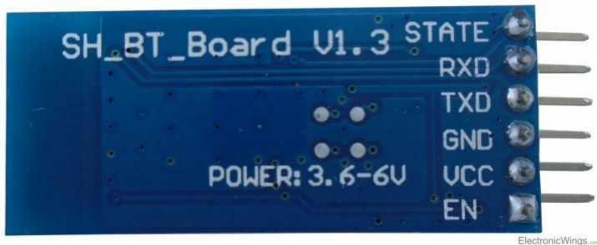
HC-05 bluetooth module pin diagram
