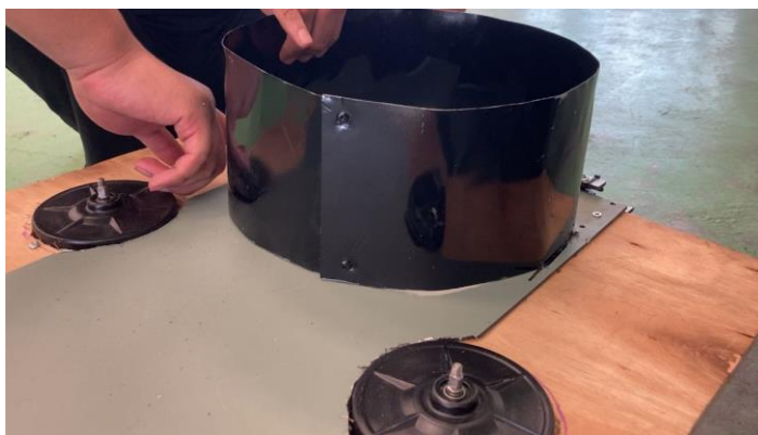
Figure 3.23: After inserting the ring loader into the passage hole, the ring loader will be fastened with a screw so that it does not come off from the hole.
