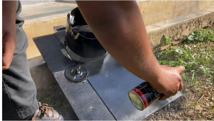
Figure 3.24: After completing the installation of the ring holder then colour the project on the top using black spray to get a beautiful colour and suitable.
