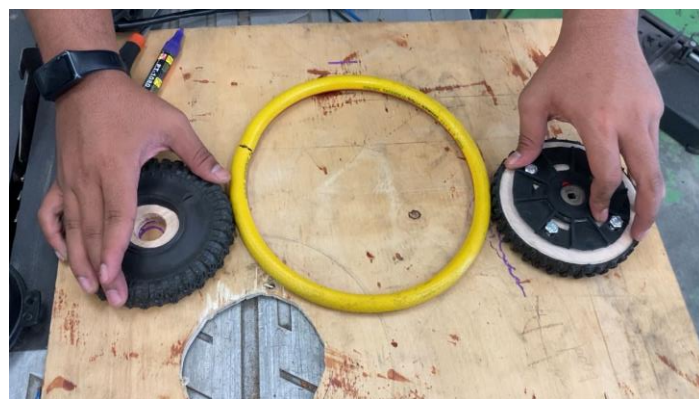
Figure 3.2: Measure the position of the motor according to the appropriate size of the ring.
