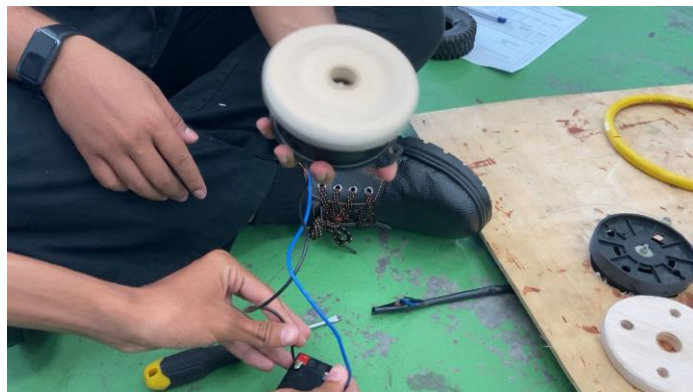
Figure 3.7: Attach the wheel to the motor to test the wheel if the wheel fits the motor.
