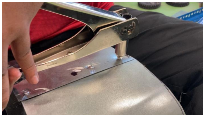
Figure 3.16: The two surfaces of the iron plate are riveted so that the iron plate sticks and becomes a permanent cylinder.
