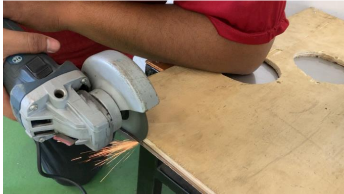
Figure 3.12: Cut the iron plate that is more than the board to get the same size by using a grinder.
