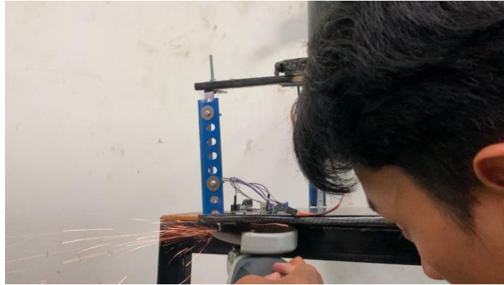
Figure 3.27: Cut off the excess screws that come out.
