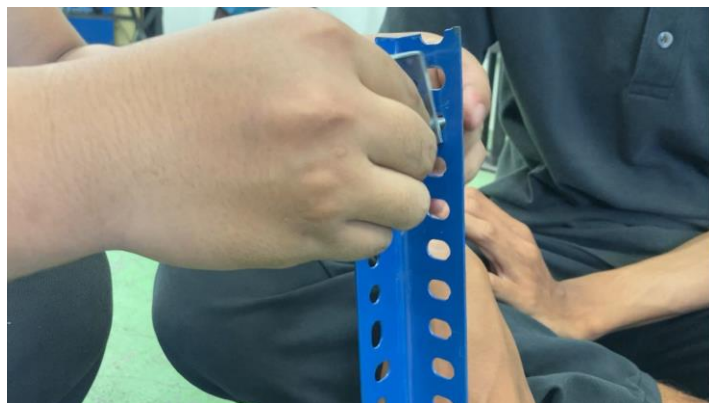
Figure 3.26: The pole is fastened to the L connector to connect the bottom and top boards into one.
