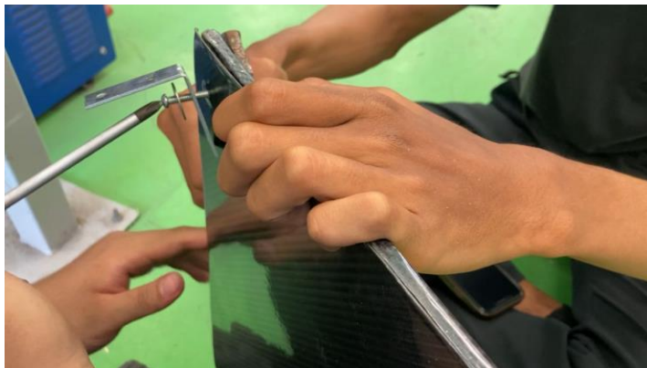
Figure 3.25: The L connector is fastened using screws at each corner of the bottom and top boards.
