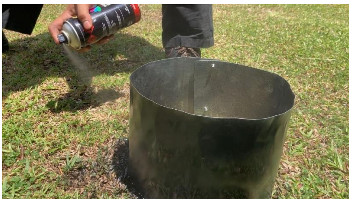
Figure 3.17: Ring loader sprayed using black spray.
