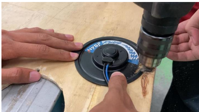
Figure 3.8: Make screw holes using a drill to fasten the motor so that the motor does not fall.
