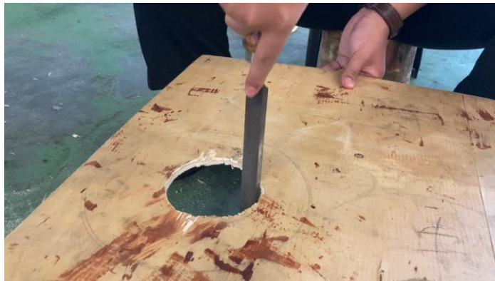
Figure 3.4: Scrape off the excess on the hole that has been made to fit the motor in.
