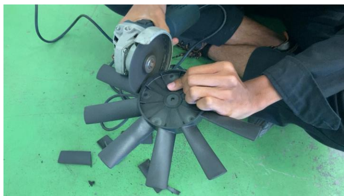
Figure 3.5: This is the process of making ring shooter wheels.
