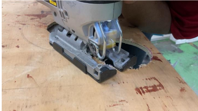
Figure 3.3: Make two holes with a diameter of 9cm to insert the motor.
