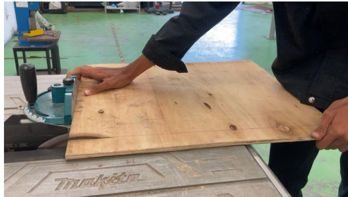
Figure 3.1: Cut two board into a size of 55cm x 60cm for base and top.
