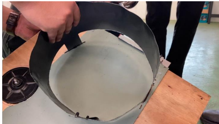
Figure 3.22: Ring loader inserted into the passage hole.
