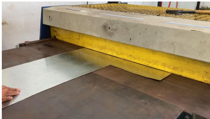
Figure 3.13: Cut the iron plate into a size of 30cm for length and 15cm for width to be used as a ring loader.
