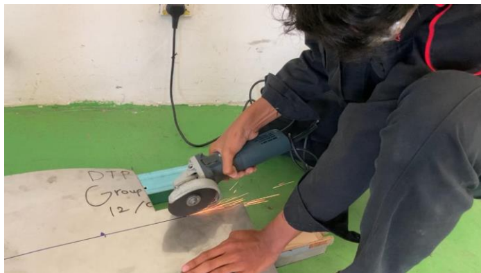
Figure 3.10: Cut the iron plate into a size of 55cmx60cm to be used as a lining for the base board.
