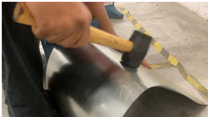
Figure 3.14: Knock the iron plate using a rubber coupling so that the iron plate is formed into a cylinder with a diameter of 25cm.
