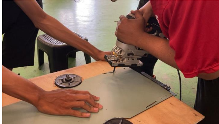
Figure 3.21: Make a passage hole to insert the ring loader.
