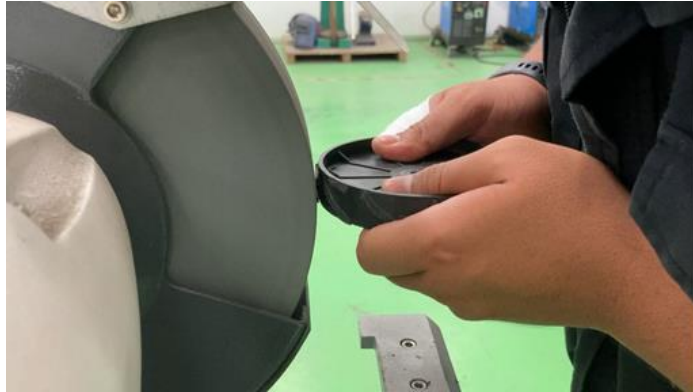
Figure 3.6: Scrape the surface of the wheel rim to make the surface of the wheel rim flat and not bumpy.
