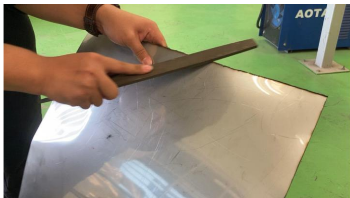
Figure 3.11: Scrape the edges of the iron plate so that there are no excess effects from the cutting done on the iron plate.
