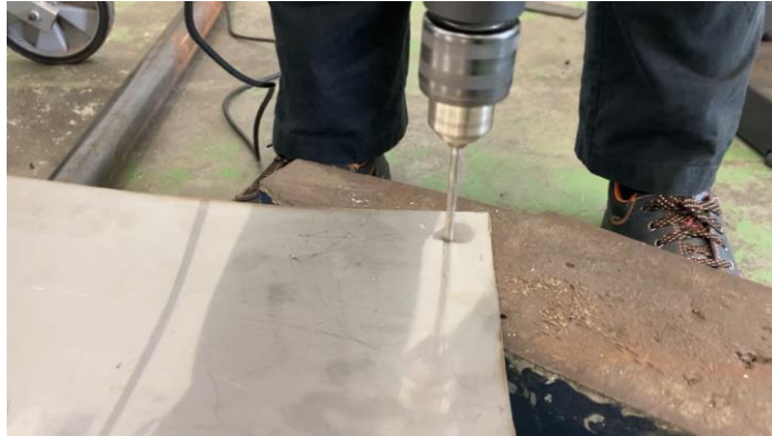
Figure 3.15: Make a hole using a drill on an iron plate that has been shaped into a cylinder to be riveted.
