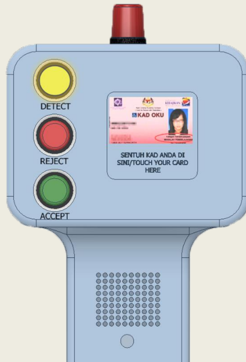
Rajah 6: Komponen utama Smart Sensor Parking for Disabled Person
