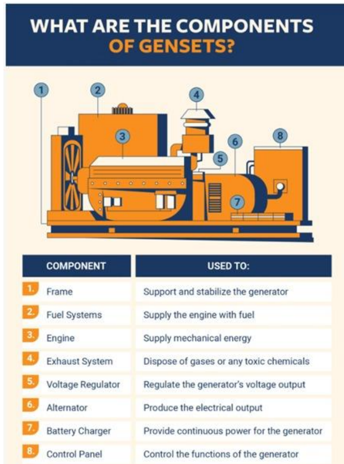
Figure 2.1: The Component of Genset (Tolbert 2003).
