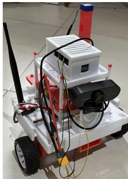
Figure 7. X-Lakbay snap-fit 3D-printed robotic platform. Cropped from [22], Figure 1A, under the Creative Commons Attribution License.
