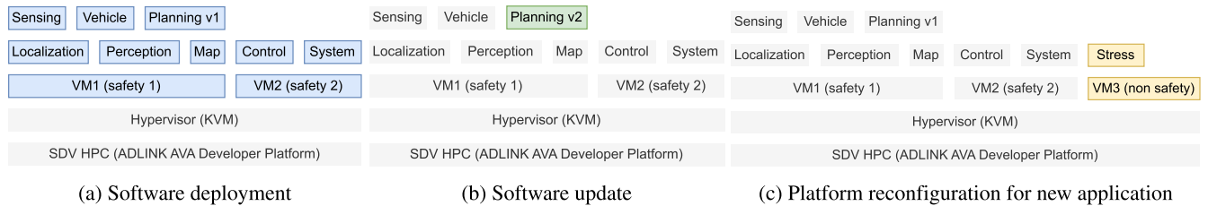
FIGURE 3. Scenarios in SDVs. The illustration of SDV scenarios is based on the demonstration setup from Section VII. (a) Eight Autoware applications should be deployed on an in-configured SDV HPC. Due to varying requirements of the applications, two different VMs should be created. (b) The application Planning is planned to be updated on the fly. (c) The platform requires a new VM to host a non-safety application Stress.
