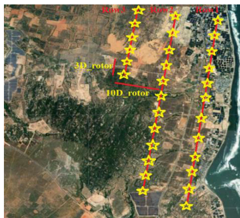
FIGURE 30. Optimal configuration for installing the E103 turbines [64].
